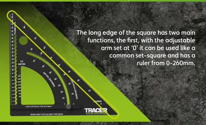
The second, like the set-square, is the ability to quickly create an angled mark. Just pivot the square using the graduations on this outer edge as a guide. You can now quickly and simply pivot the square to mark any angled cuts from 0°-90°.
