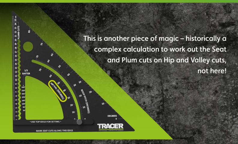
Again, simply set the HIP/VALLEY scale to the pitch of the roof and the square is set up for marking your Seat/Plum cuts on your Hip and Valley rafters – simple as that.
