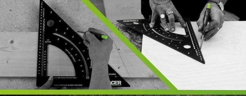
"Very simple to use. Just need to set the scale to whatever the roof pitch is and mark your seat and plum cuts for either the Jack and Com or Hip and Valley cuts!"
